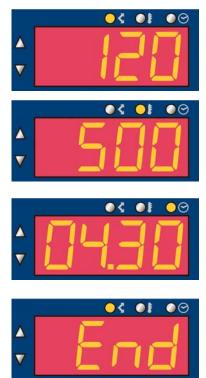
Explanation: the full range of displayed values for ramp rate are: End, 1...999°C/hr, FULL. To mark the end of a program select a ramp rate of "End" by holding down the **DOWN** key until End is displayed. To add an extra segment press the **UP** key until your desired ramp rate is shown. If you want to heat at full power hold down the **UP** key until FULL is displayed.
