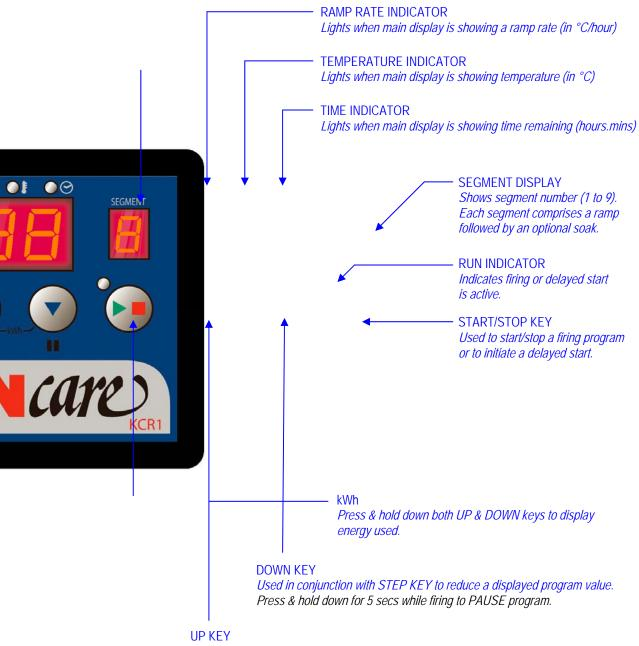
Used in conjunction with STEP KEY to increase a displayed program value. Press & hold down for 5 secs while firing to ADVANCE program.
